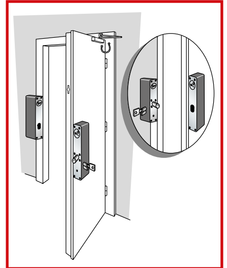
VERTILOCK for surface mounting on the doorpost or the counterframe.
